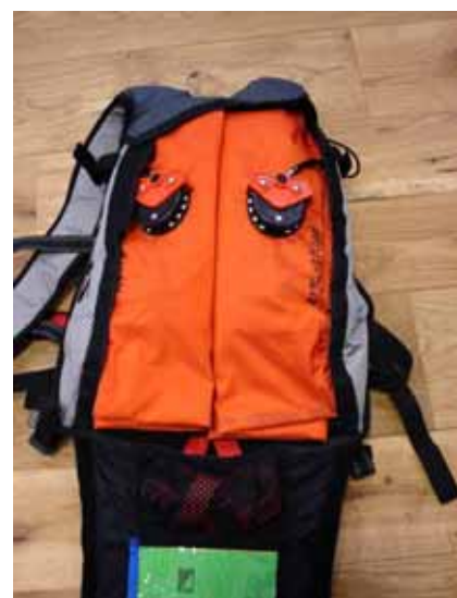
9. Fully packed Freeride backpack. Please note the correct positioning of the black and red plastic bases with the release valves. The airbags should be folded to the correct full internal length of the backpack.
