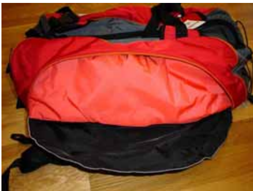
13. Fully folded and packed airbag before final closure of the Velcro cover panel
